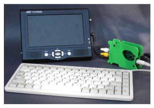
The handiwork of Human Informatics, the Reader is designed for homes and <u>schools</u> that have no budget for PCs and no internet connection for downloading content. It's built using three Atmega328p microcontrollers complete with an SD card reader and microUSB port; display output is via a composite video port. There's also infrared support, audio and four hardware buttons.
